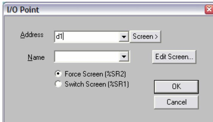
From this configuration box, there is the added ability to click the ‘Edit Screen...’ button and go directly to the screen editor for the screen specified. There is also an option of using this coil to Force the screen or Switch the screen.
