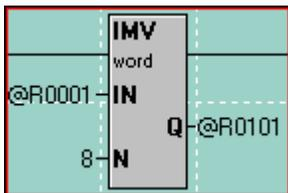
In this example, the Mother of All Confusion, both the IN and the Q are specified as Indirect. This means the controller will look at %R1 and see a value. Let's say it is 241. The controller also looks at the value in %R101. Let's say it is 341. The controller will then take the values in %R241-%R248 and move them into %R341-%R348.
