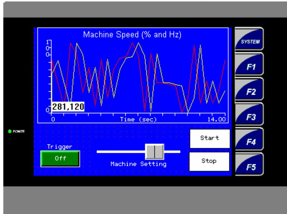
This screen adds “Start” and “Stop” capabilities to this screen. The “Start” and “Stop” Static Text legends on the above screen are only that – legends for the function keys next to them. The user must press F4 to activate the Start Functionality, and F5 to activate the Stop functionality. Use the same Start (%M1) and Stop (%M2) bits previously assigned.
