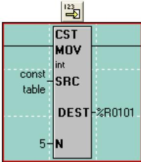
Skipping to the 'Constant Move', or 'CST MOV', it is used to move a group of constant values into a group of consecutive registers. If, for example, you want to move the values 1, 2, 3, 4 and 5 into %R101, %R102, %R103, %R104 and %R105, respectively, then you can use the Constant Move function. The count (N) is automatically determined by how many constant values you enter into the configuration for this function. The source data can ONLY be constant data and cannot be register references.
