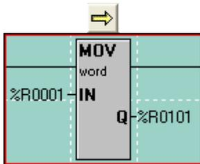
The first type of Move is the 'Move Word', or 'MOV'. It is used to copy a single byte, word or double-word from one location to another. The count is locked at 1. In the case of the example to the left, the value in %R1 is copied into %R101. This only happens when the ladder rung receives power. The value in %R101 is NOT taken back out when power is lost to the rung. The IN can be either a register or a constant value.
