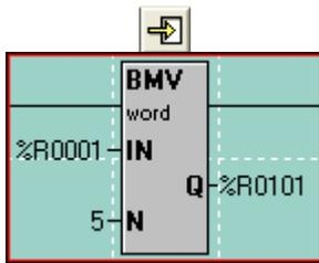
The next type of Move is the 'Move Data Block', or 'BMV'. It is used to copy a group of bytes, words or double-words to another location. The count (N) determines how many registers are to be copied. In the example to the left, %R1-%R5 are copied into %R101-%R105. Again, this only happens when the ladder rung receives power. The IN must be a register reference and constant values are not allowed.
