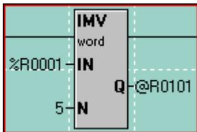
In this example, the Q is specified as Indirect. This means the controller will look at %R101 and see a value within it. If %R101 has a value of 851, the controller will take the data in %R1-%R5 and move it into %R851-%R855.
