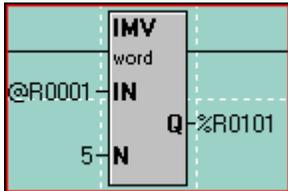
In this example, the IN is specified as Indirect. This means the controller will look at %R1 and see a value within it. If %R1 has a value of 501 in it, the controller will go to %R501 to get the source data. 5 registers will then be moved from %R501-%R505 to %R101-%R105.
