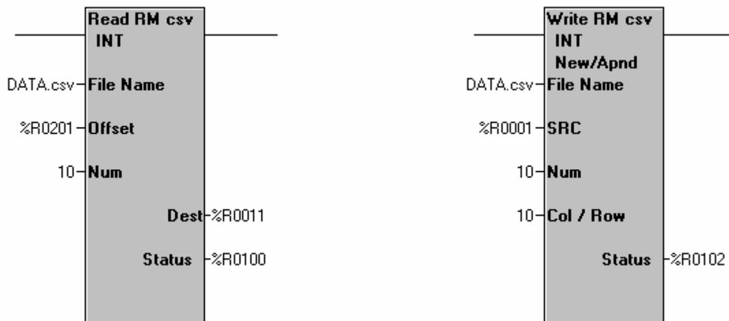
1. Open Cscape and create a ladder program that will write 10 registers of information, starting at %R1, when triggered by %T1. Use the Write RM function configured for Create/Append to perform this action and call the file Data.csv. Place a rest coil after the Write RM function with the address of %T1.
